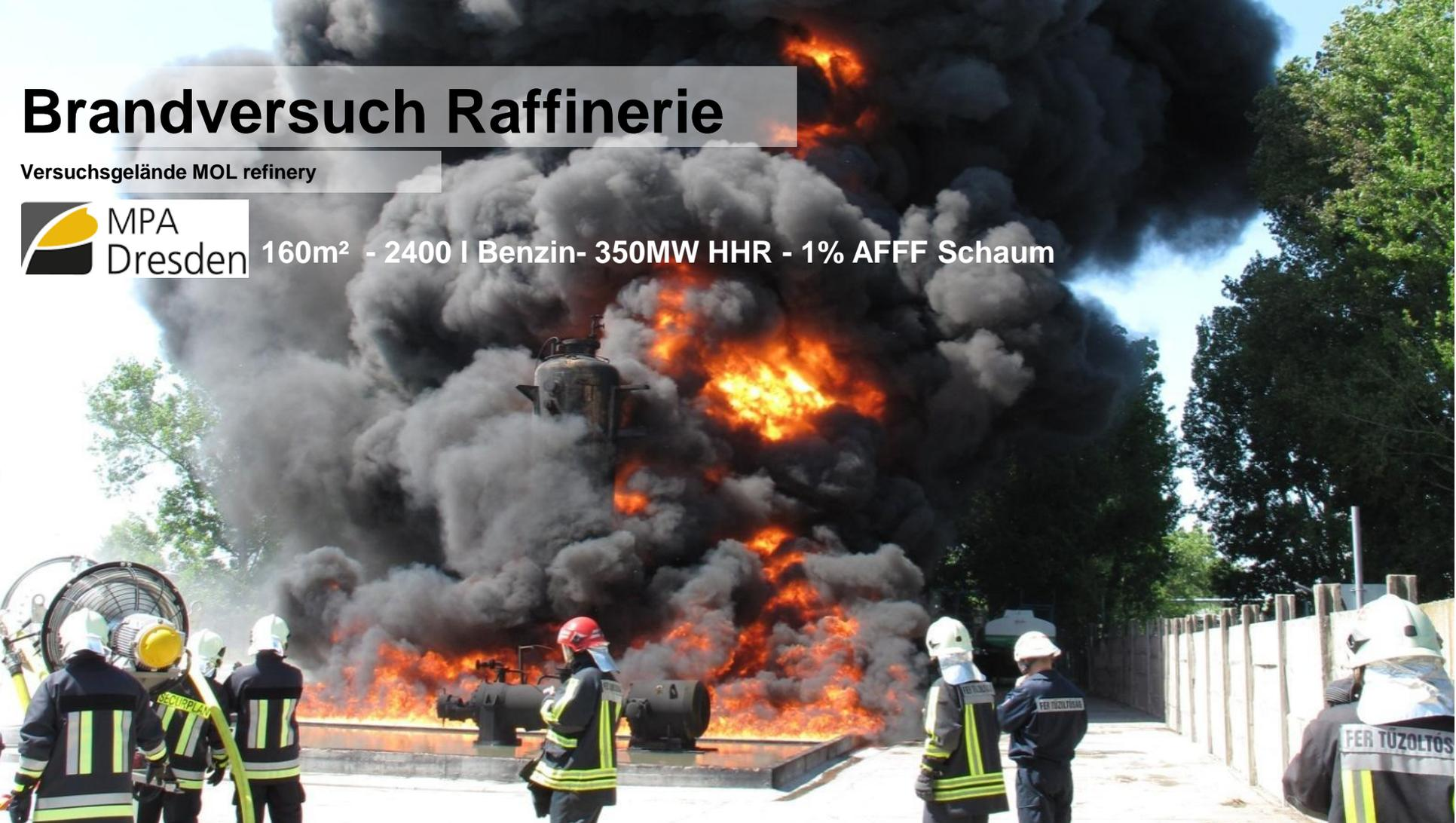
**Test:** 160m<sup>2</sup> - 2400 l Benzin- 350MW HHR - 1% AFFF Schaum
